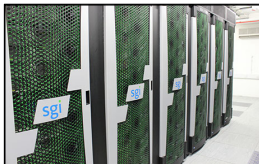
SGI UVs 2500 cores 20 Tbytes RAM
